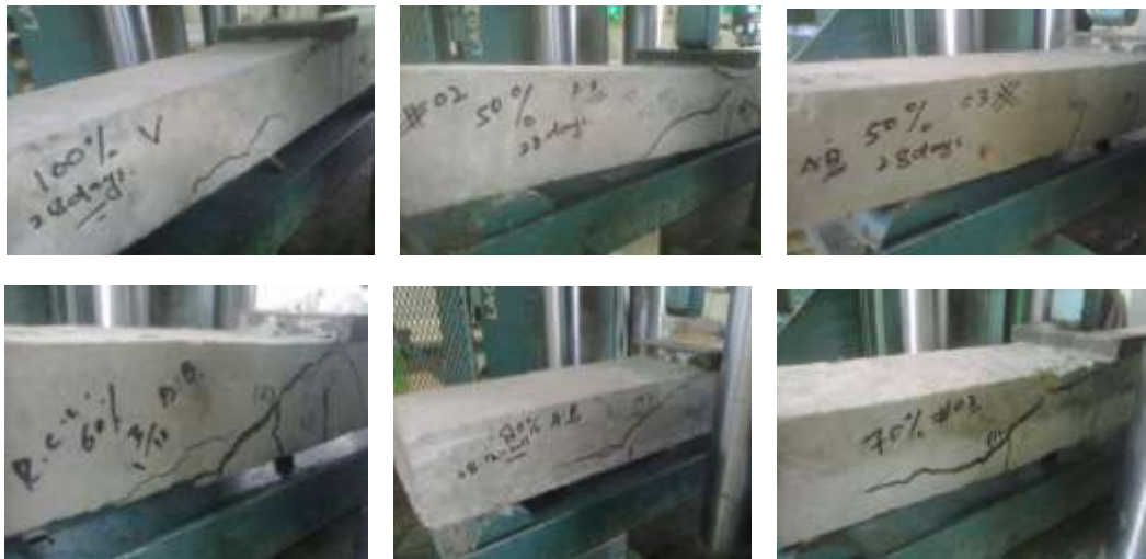
Figure 10: Cracking in slabs for selected models
